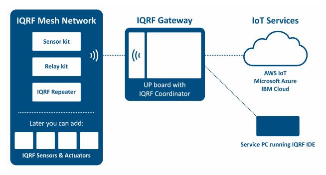
UP board is connected to the IQRF network via SPI interface (adapter) or via CDC interface (GW-USB/CK-USB).
